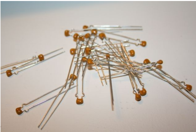
14. Solder 20pF capacitors.
