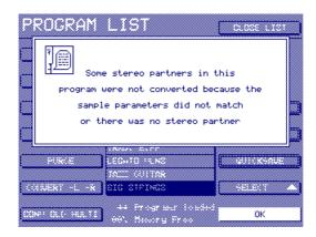
You should press OK and identify those samples that do not match and make the necessary adjustments.
