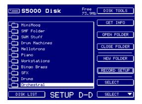
You can use the SELECT keys (F15/16) in conjunction with OPEN and CLOSE FOLDER to navigate your way around the folders in the filelist to select where the new disk recording will be recorded to. Alternatively, you can create a new folder to record to.
