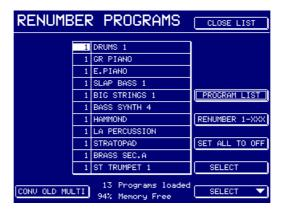
In either screen, you can convert such a setup simply by moving the cursor to any program sharing the same program number and pressing CONVERT OLD MULTI. You will receive this prompt:
