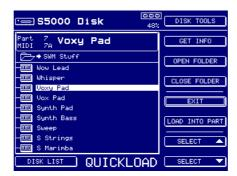
As you can see, the program VOXY PAD is now loaded into Part 7. A feature of QUICKLOAD is that you may immediately audition this sound by sending MIDI data on the appropriate channel. If the sound is not to your liking, you can repeat the QUICKLOAD procedure until you find a sound you like. Once you have settled on a sound you like, if you return to the main MULTI page (either by pressing EXIT - F13 - followed by CLOSE TOOLS or more directly by pressing the MULTI mode key), you would see this:
