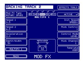
SPEED 1 This sets one of the rotary speaker speeds. Typically, this will be used to
