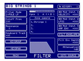
The filter plays a key part in any sound and is responsible for some of the most dramatic real-time effects available on the S6000. Amplitude can change level and panning can move the sound around in the stereo image and, of course, you can add vibrato from LFO 1. The filters, on the other hand, can totally transform a sound (especially with 26 to choose from!). So, before we look at the various parameters, what is a filter?
