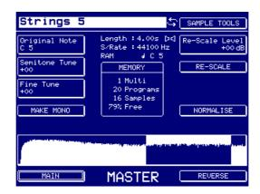
The sample's waveform is shown at the bottom of the screen. The inverted/highlighted area is the sample's loop.
