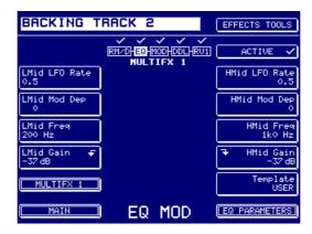
The LOW MID and HIGH MID bandpass filters of the EQ are able to be modulated by their own independent LFOs. The LMID and HMID LFO RATE parameters set the speed of these LFOs and the LMID and HMID MOD DEPTH parameters set the amount of LFO modulation. In this page, because there is a certain degree of interaction between the modulation and the LMID and HMID frequency and gain settings, the LMID EQ controls are duplicated here for convenience to save you swapping between pages
