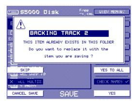
Pressing YES will replace the item on disk with the item you are saving. Pressing SKIP will keep the original on disk and will not save the new item.
