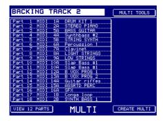
Here you can see each part has its own MIDI channel (VIEW 18 PARTS is shown here to make the example clearer).
