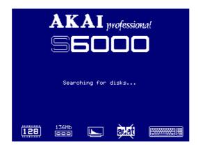
The icons appearing at the bottom of the screen indicate what hardware is installed.
