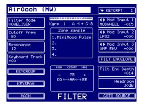
Two examples of vowel filters to produce vowel articulations as described in their program names. The modwheel controls the effect.
