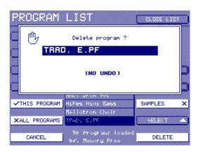
The SAMPLES checkbox on F14 allows you to select whether you also want to delete the samples associated with the selected program. With it checked, the samples will be deleted.
