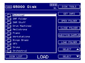
The folder MUST be in the root directory and not buried in another folder. It can use any combination of 'case' and "AUTOLOAD", "Autoload", "AutoLoad" would be valid. However, "Auto Load" or "Autoload 1" would not.
