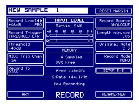
However, before you make a 'virtual' recording, you need to select *where* on the disk you are going to record to. This is done in D-D SETUP (F14) which will display something like this screen:
