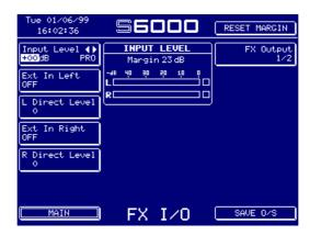
It is possible to use the EB20 as an effects processor for external signals fed into the sampler's inputs (the EB20 is an option on the S5000). An effects channel may share an external input AND internal sounds. For example, you may route some parts to FX channel 1 which also has an external input routed to it. If you want an FX channel for exclusive use by an external sound source, do not route any parts to that FX channel. The parameters in the FX I/O page are:
