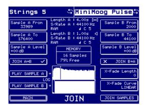
This (and MIX described next) are the only two sample editing pages that don't conform to the normal page layout due to the fact that you are working with two samples.
