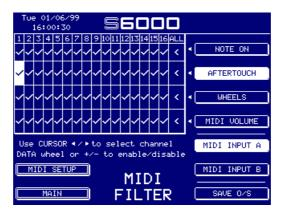
This page allows you to selectively filter out certain types of MIDI events on selected MIDI channels. This can help to reduce bottlenecks at the MIDI inputs and therefore help to keep note-on delays to a minimum.
