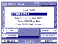
The 'check boxes' on F6, F7 and F14 allow you to disable certain items from loading. For example, you may just wish to load only the programs and samples from a folder in which case, you could disable the loading of multis by pressing F6.
