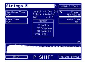
This process is a variation on timestretch. However, the 'stretch factor' in PITCH SHIFT is described in terms of transposition. For example, if you have a sample in the key signature of C which you want to use during a key transposition of a song where everything is transposed up a tone to the key of D, set a SEMITONE TUNE value of +02 semitones.
