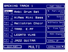
The part's parameters appear down the right hand side of the screen where you may set level, output assign, FX send level, etc.. The logic for selecting parts is as follows:
