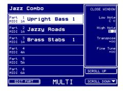
In this example, UPRIGHT BASS could be set to cover C1-B2 with JAZZY ROADS PNO set to cover C3-E5 with a handful of BRASS STABS on F5-C6. The same technique could be used in a string section setup to have cellos in the bottom octaves and violas/violins in the top octaves. Again, each 'element' in the keysplit may be routed to separate outputs and/or the effects for greater flexibility.
