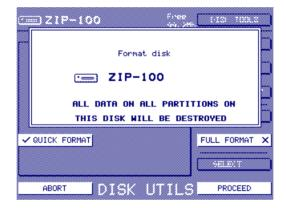
You should select whether you want to perform a QUICK FORMAT or a FULL FORMAT using the check boxes on F6 and F14. FULL FORMAT is required if the disk is brand new or has maybe been used with some other device (for example, a disk that may have been used on an older Akai sampler). The FULL FORMAT takes much longer of course but sets the disk up properly. QUICK FORMAT can be used if you are re-formatting an existing MS-DOS disk.
