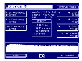
Here you have access to three bands of parametric EQ. Each band has variable frequency and gain and the 'window' function in the GAIN parameters down the right hand side of the screen offer further functionality.
