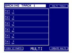
The new multi is initialised and Parts 1-16 are assigned to MIDI channels 1A-16A and Parts 17-32 are assigned to MIDI channels 1B-16B. If you created a 64 part multi, parts 33-48 will be assigned to MIDI channels 1A-16A and parts 49-64 will be assigned to MIDI channels 1B-16B. A 128 part multi will be similarly assigned. You may now fill those parts with sounds to play.
