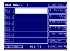
The cursor moves to the program name field. Now simply rotate the DATA wheel to scroll through the programs that are in memory until the one you wish to assign to the part is selected.
