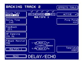
The parameters are identical to those found in the mono delay effects except that because two delay lines are used, delay time is halved (to 335mS).
