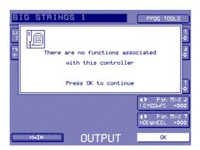
Similarly, if the mod source is one of the MIDI controllers (pitchbend, modwheel, keyboard, etc. - in other words, a controller that has no parameters associated with it), you will receive the same prompt.
