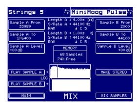
As in JOIN, use F1 and F9 to select the samples you want to mix. The process will merge the two samples, effectively 'layering' them into one composite sample.
