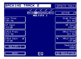
The EQ section of the two multi-effects channels is a four band EQ offering lowpass control over a low frequency, two bandpass mid frequencies and a highpass high frequency control. I.e.:
