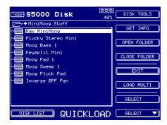
This is showing you all the multis in a folder called "MINIMOOG STUFF" which is on a removable hard disk called "S5000 DISK". You may close the currently active folder and select and open a different one and/or you may also select another disk to load from using DISK LIST on F8.
