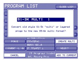
Press ADD TO CURRENT to add the selected program number to the currently selected multi or press CREATE NEW to create a new multi to add the program(s) to. If you create a new multi, its name will be that shown in the prompt (i.e. S1-3K MULTI 1).
