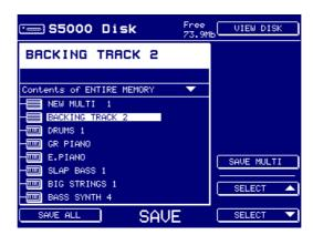
In this example, you were working on the multi BACKING TRACK 2 when you pressed SAVE. This is therefore the item selected to save. Had you been working on a sample or a program, the appropriate item would be shown to be saved.
