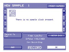
You should either record via the analogue inputs or connect the appropriate digital device.
