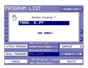
The SAMPLES checkbox on F14 allows you to select whether you also want to delete the samples associated with the selected program. With it checked, the samples will be deleted.
