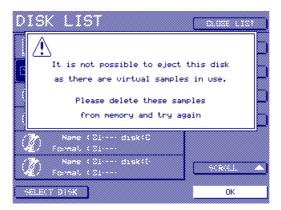
You should press OK and, in EDIT SAMPLE, identify the 'virtual' samples in memory and delete them. Once all the 'virtual' samples from the selected disk are deleted, you can eject the disk as usual from its own front panel.
