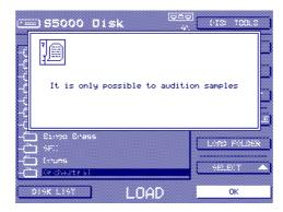
When you press AUDITION SAMPLE, there will be a small delay as the sample is found on disk and played out. You should press *and hold* the AUDITION SAMPLE key until the sound is played.
