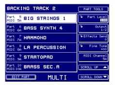
In this situation, you can use the SCROLL UP/DOWN keys to select another part if you wish to edit the same parameter for that part. For example, if, in the above screen shot, you wanted to balance the levels for Parts 6, 7, 8, etc., you could use SCROLL DOWN very effectively:
