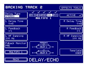
The parameters are identical to those found in the mono and crossover delays except that you have independent control over both channels delay time, feedback and HF damping. The PING PONG parameter is not available in this delay effect type.
