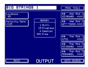
This page sets parameters that affect the final output level and pan position of the program. The parameters are:
