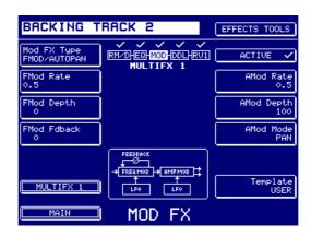
This effect type allows you to modulate frequency and/or amplitude for a variety of vibrato, autopan, tremolo and Doppler Shift effects. The parameters are:
