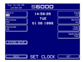
The time you entered this page is captured in the centre of the screen (the actual time the sampler was previously set to keeps ticking away in the top left corner). You should set the various parameters accordingly to set the time and date and, at an appropriate moment, press SET (F16) to actually set the time.
