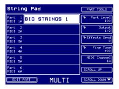
The MULTI mode can be used to play single programs simply by assigning just one program to a part. In this way (especially with 128 multis available), the S6000 can be used as a simple playback module for playing single sounds.
