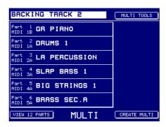
In this example, the GRAND PIANO is the part you would play live through MIDI input B whilst the other parts are sequenced via MIDI input A.
