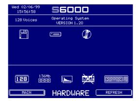
At a glance, you can see how many voices are available to you, how much memory is installed, whether the effects processor EB20 is installed (S5000 only), whether the ADAT option is fitted, whether the keyboard is attached and what drives are connected. Those items shown with a cross through them indicate that they are not installed/attached.
