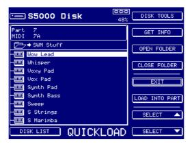
The QUICKLOAD screen is much like the normal load page except that, because you cannot load samples or multis into a part, you only see the programs in the selected folder.
