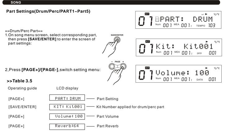
3. Press [+]/[-] or DIAL to adjust settings of the corresponding parameters.
