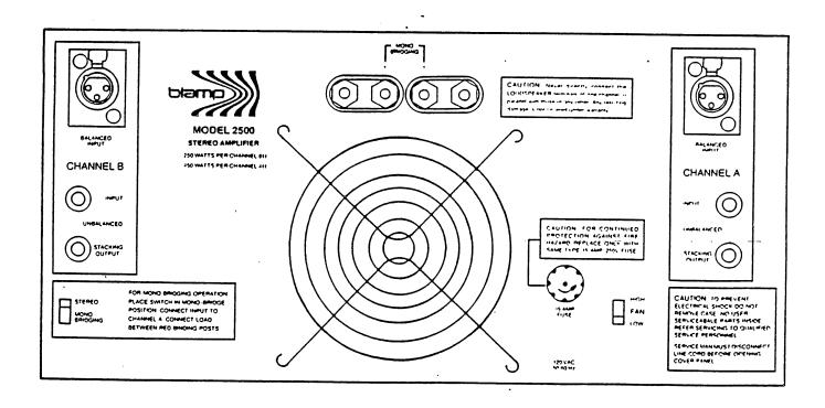
When using the balanced XLR input, the output impedence of the stacking output jack is 1000 ohms. Up to 20 amplifiers can be driven when the balance input is on the initial amplifier.
