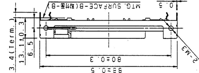
MOUNTING HOLE DETAIL (取付穴寸法)
