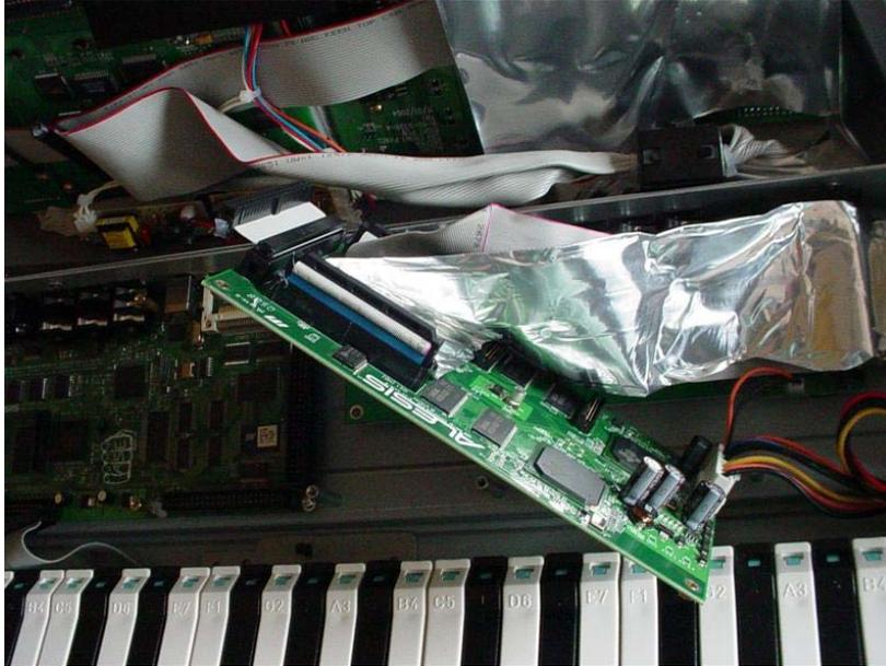
If you look closely you will see that there are many ribbon cables and power cables still attached to this board. You do not want to rotate this board too far or you may disconnect or even damage one or more of the cables. Looking further back towards the back of the board you can see the SDRAM Expansion slot underneath the metallic tape/IDE cable:
