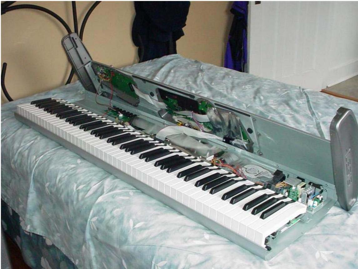
It is a good idea to put something else in place to brace the assembly so it does not tilt all the way back or shift around during the remainder of the process. I put a pillow behind it...
