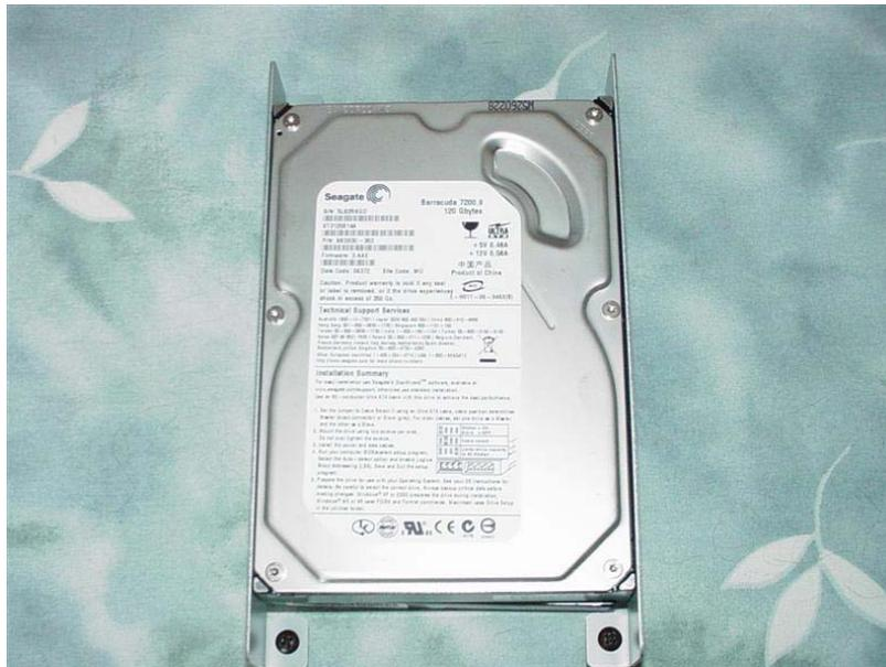
Re-mount the hard drive assembly back into the Fusion chassis using the 4 black screws making sure that the drive faces the correct direction (cable sockets on the left-hand side).
