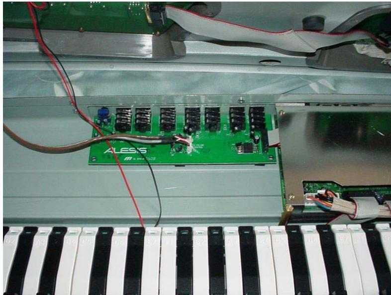
The Mainboard housing (covers the mainboard and expansion board):
