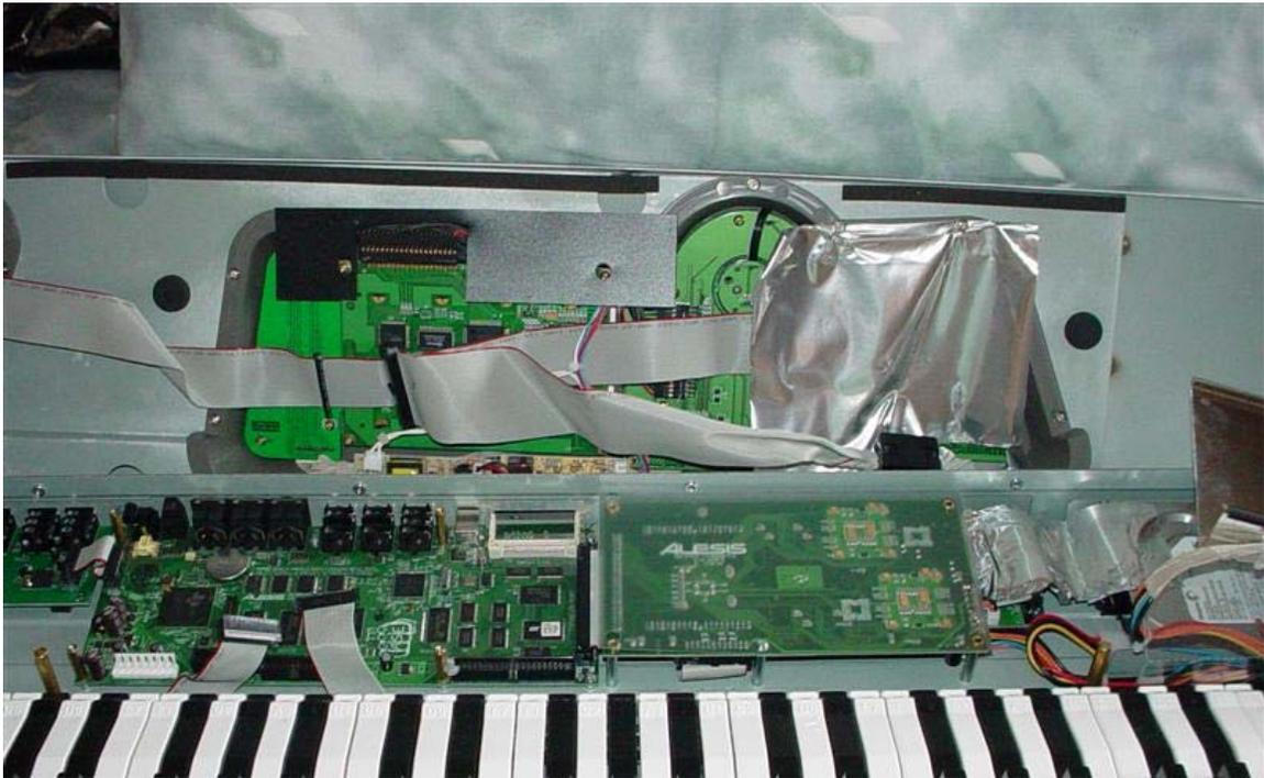
You will now see the mainboard (on the left side) and the expansion board (right side – shows the ALESIS logo in white). You should have two E3 modules – one module goes on each of these boards.
