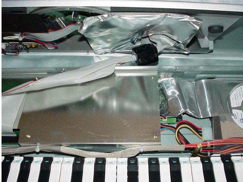
The Hard Drive assembly (note the clear plastic cover slip over the power cables):
