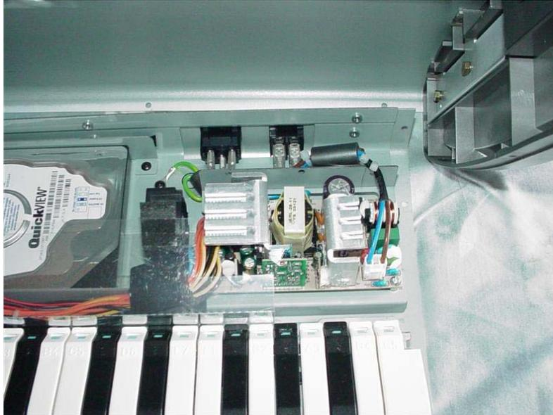
Now that you have an idea of what is where inside of the Fusion, move on to the next applicable step for you. The hard drive installation (Step 4) is what I did first and this is the easier of the two upgrade activities. If you are not installing a hard drive, skip to the E3 Memory Module Upgrade in Step 5.
