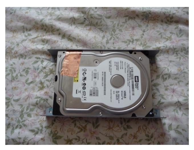
Next, remove the screws holding the drive to the cradle parts and set the HDD to one side.
