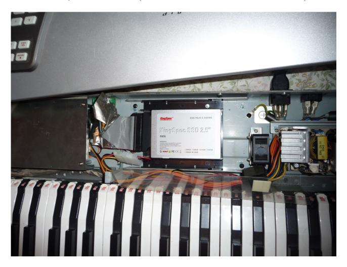
The SSD arrives set to "Master" as shown below, and I installed it "as received".
