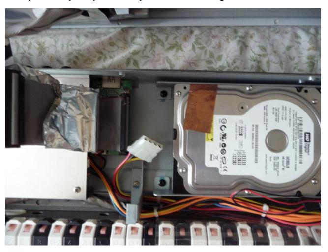
I have unplugged the data ribbon and the molex power to show the BLACK screws that hold the HDD's cradle to the base of the Fusion.
