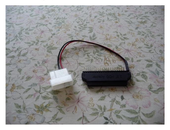
The 3.5" "side" has ALL pins present, unlike the outgoing HDD which has one pin MISSING.
