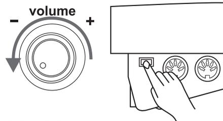
Set the power switch to "on" position to switch on the power. Display shows the kit's number and its indicator lights up.
