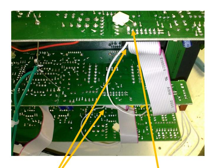
Separate the last conductor from the 16way IDC and pull away from rest of harness.
