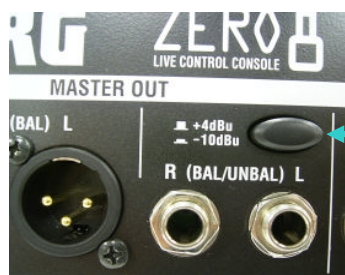
MASTER OUT(TRS) +4dBu/-10dBu SWITCH
